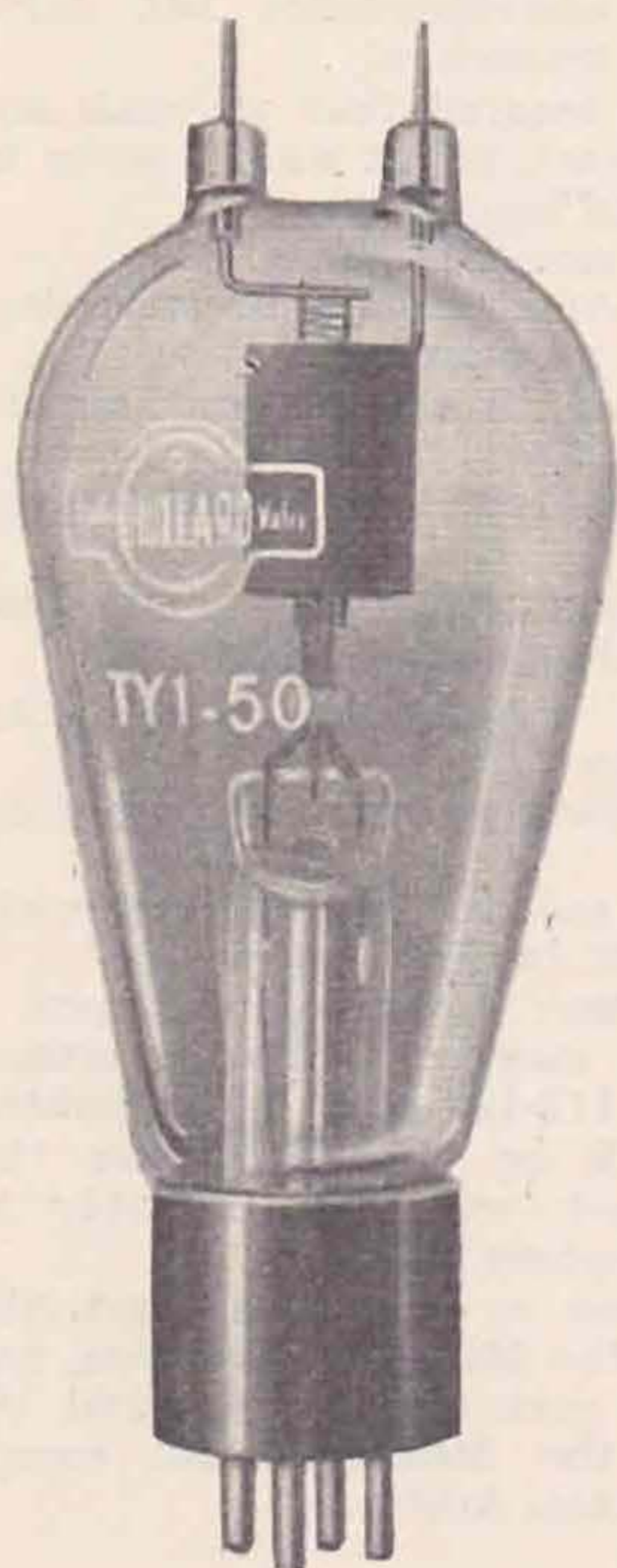
The Mullard TY1-50, an efficient Triode up to 150 Mc.
